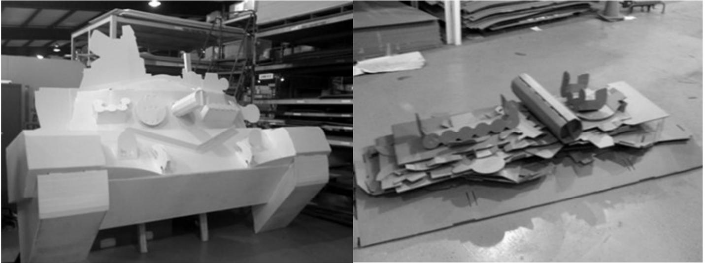
**Figure 7: RLCT T-72 Frontal Target: Assembled, and Knocked Down Flat for Shipping**
