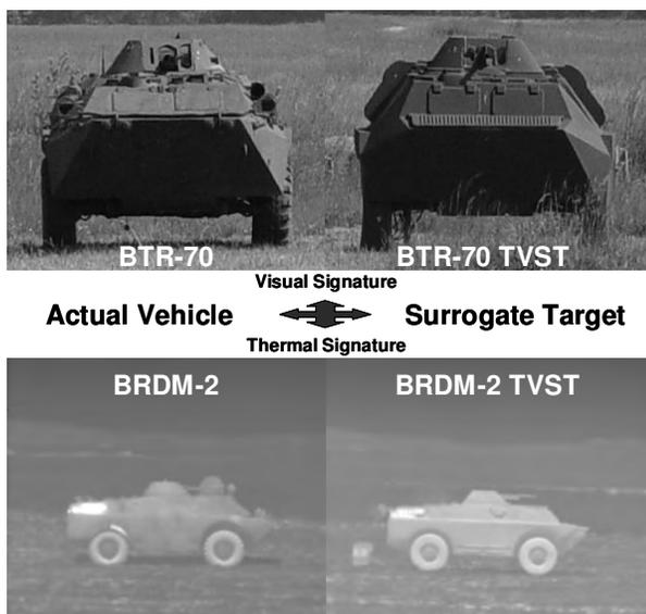
**Figure 2: TVST 2.5-D Visual and Thermal Signature Comparison to Actual Threat Vehicles**
