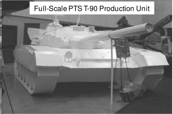
**Figure 5: Full-scale PTS T-72 and T-90 Targets**
