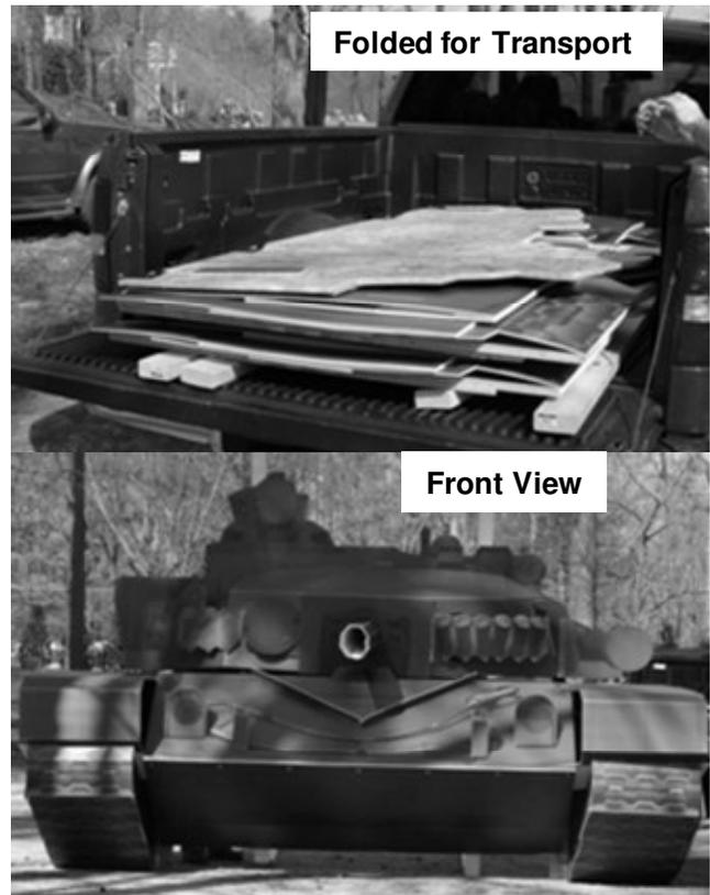
**Figure 4: Full-Scale PTS T-72 2.5-D Frontal Target**
